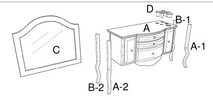
Once the legs are firmly attached, replace the drawers and carefully flip the station back over so it is right side up. It would be very beneficial to have another person help, with each person on either side. This would greatly reduce the risk of dropping the station and reduce any strains on the legs.
